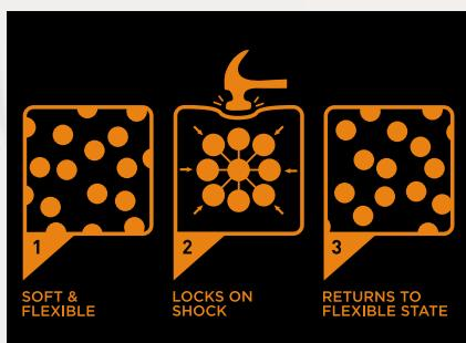
**High-tech D3O® material.** D3O® is an active and specially engineered material made of intelligent molecules. They flow with you as you move, but on shock they lock together to absorb the impact energy.
