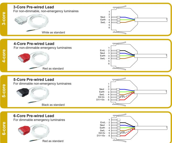
Note: Ordinarily, plugs used in the manufacture of pre-wired leads are only fitted with sufficient pins to suit the lead\*
